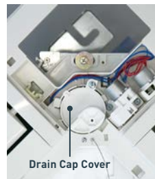
Remove drain cap cover and check the condition. To clean, firstly remove the rubber plug to drain water before removing the drain cap.
